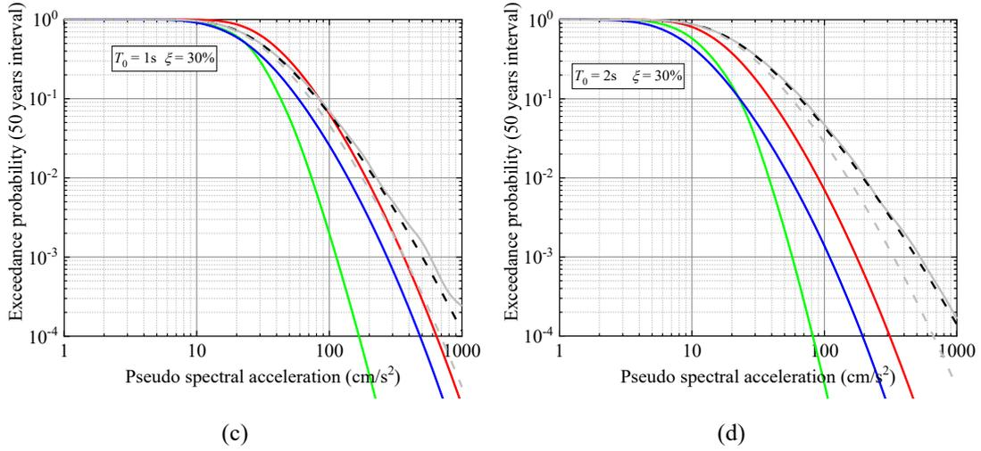
594 Fig. 8 Exceedance probabilities of the PSA at 50-year intervals for a 30% damping ratio obtained using
