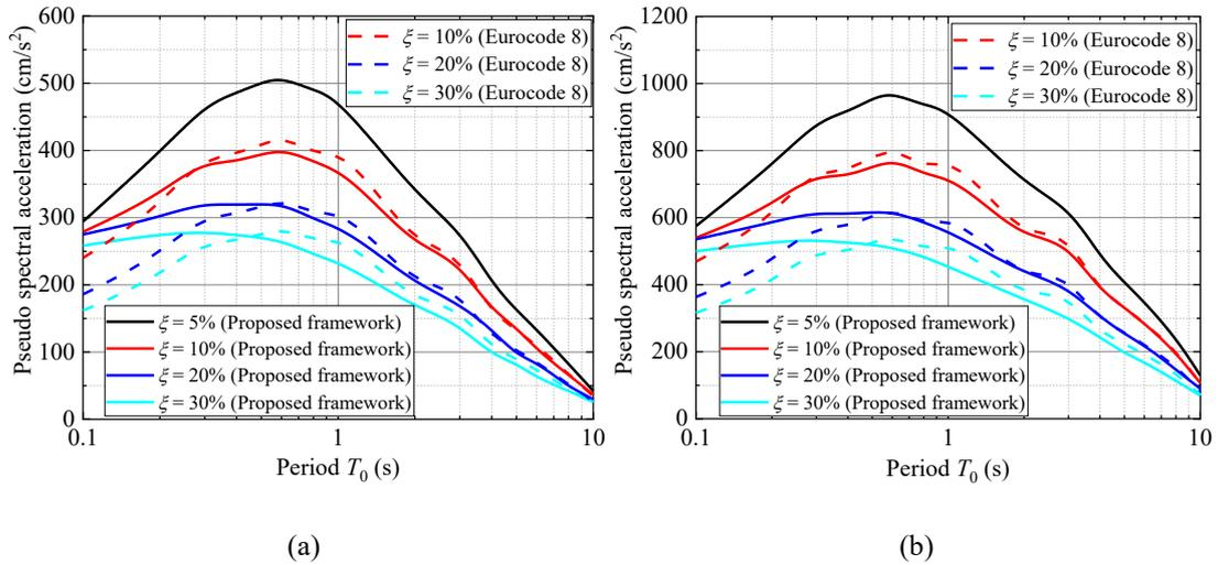
605 Fig. 11 Comparison of uniform hazard spectra for different damping ratios obtained using the proposed
