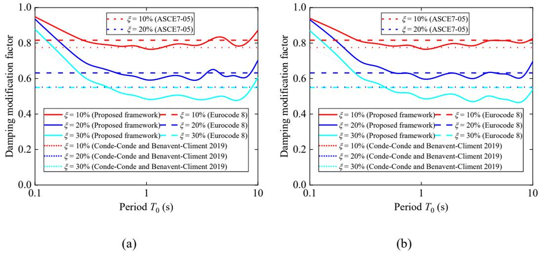
612 Fig. 13 Comparison of damping modification factors obtained using the proposed framework and the
