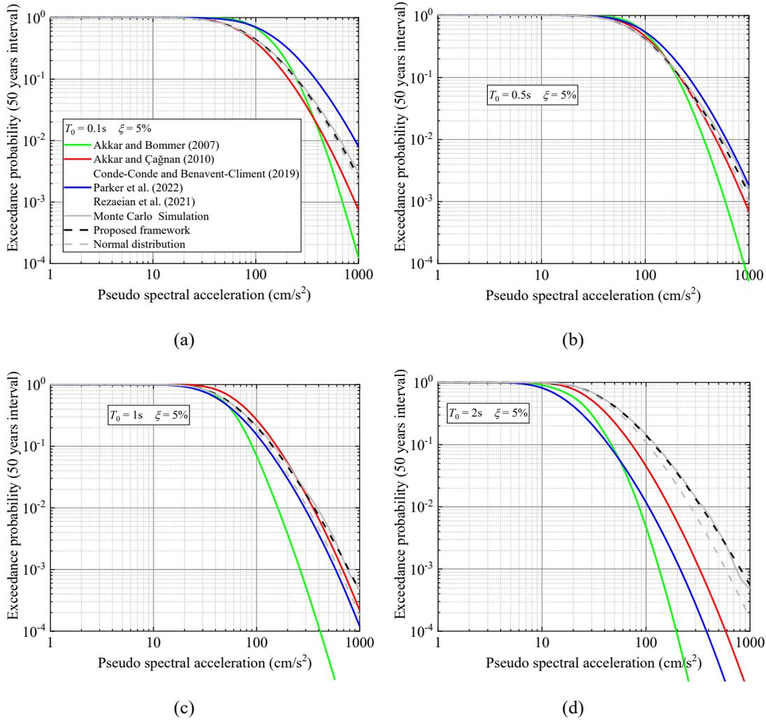
586 Fig. 6 Exceedance probabilities of the PSA at 50-year intervals for a 5% damping ratio obtained using
