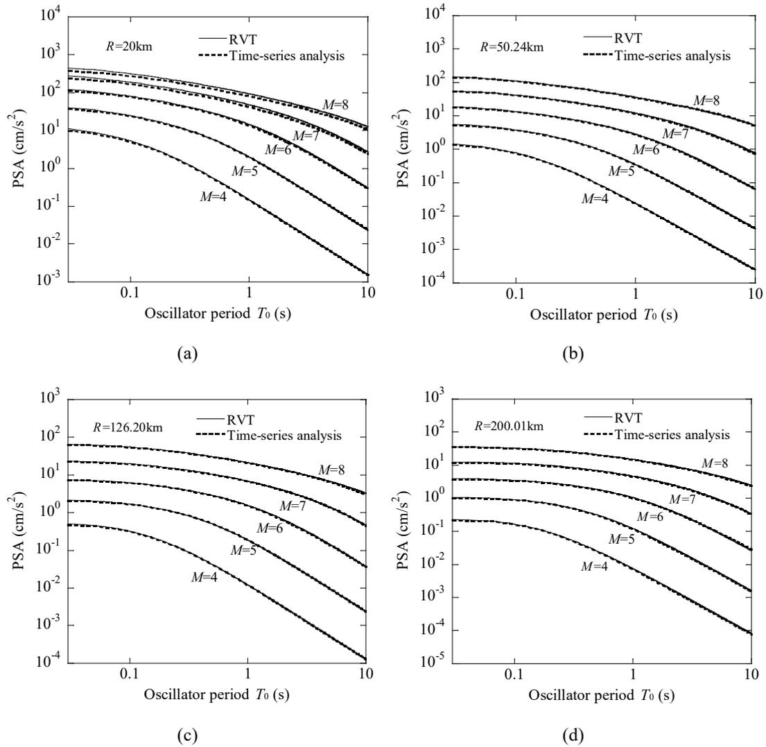
576 Fig. 3 Comparisons of PSA results for a 50% damping ratio calculated using Eq. (5) and time-series
