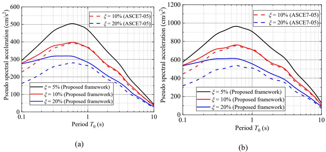
609 Fig. 12 Comparison of uniform hazard spectra for different damping ratios obtained using the proposed
