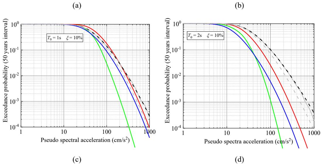
590 Fig. 7 Exceedance probabilities of the PSA at 50-year intervals for a 10% damping ratio obtained using
